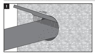
Clean the plastic pipe in the area where the Hilti Firestop Wrap CFS-W is to be installed.1
