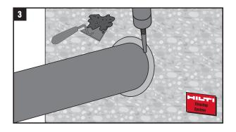
Seal the remaining gap with Hilti Firestop Acrylic Sealant CFS-S ACR or a cementitious mortar. Use minimum 25 mm Hilti Firestop Acrylic Sealant CFS-S ACR in case of flexible wall constructions, minimum 15 mm in rigid wall constructions and minimum 10 mm, backfilled with mineral wool, in case of rigid floor constructions. In case of use of mortar the gap is to be filled completely over the entire thickness of the wall or floor.
