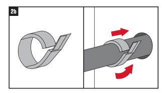
Cut the Hilti Firestop Wrap CFS-W EL to length according to the outer diameter of the pipe, taking the required number of layers into consideration. If sound decoupling means are installed around the pipe this has to be considered when cutting the wrap to length. Wrap the Hilti Firestop Wrap CFS-W EL around the pipe and secure it with a short strip of adhesive tape. Push the Hilti Firestop Wrap CFS-W into the annular gap until its outer edge is flush with the surface of the wall or floor.
