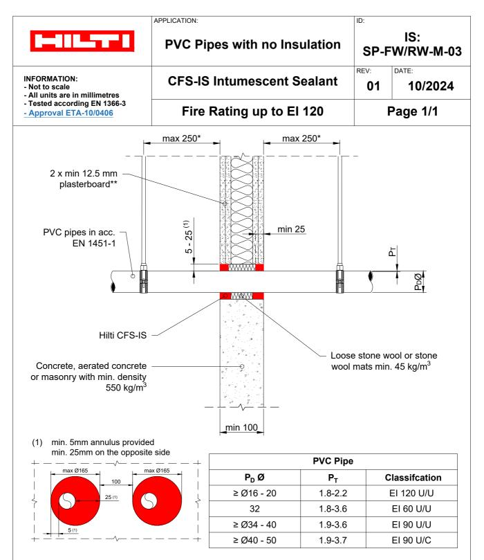
Max opening size 150mm x 150mm or circular openings of equivalent area ( $\emptyset$  165mm). Min. 100mm distance to other firestopping penetrations and timber studs. Min. 200mm to other penetrations (e.g., doors, windows etc.)
