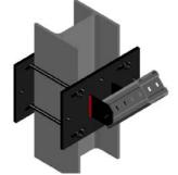
3. Base plate and through bolts - per analytical calculation
